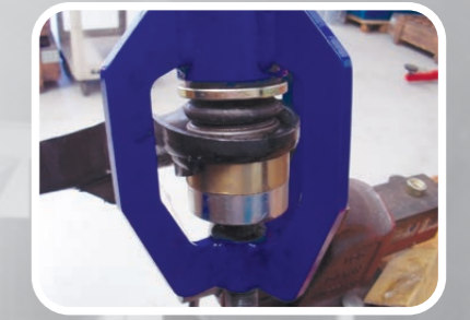
Installing Navara Ball Joint
