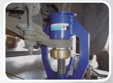
Installing Ford Bottom Ball Joint
