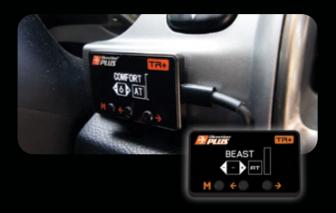
The Direction-Plus™ TR+ Throttle Controller is a compact unit that will increase throttle response by adjusting the signal sent to the vehicles ECU and eliminating throttle lag, giving you more response!
