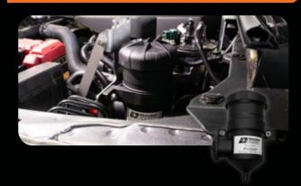
The Direction-Plus ProVent Ultimate Catch Can kits separate oil from the blow-by gases by means of an oil separating element, reducing the amount of oil in the blow-by gases returning to the engine.
